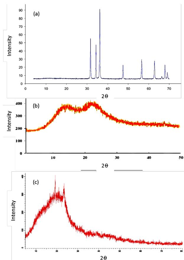
Fig. 6. XRD pattern of (a) Commercial ZnO nps (b) Paint (c) ZnO-APO paint.
