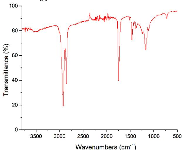
Fig. 3. FTIR spectrum of APO.
