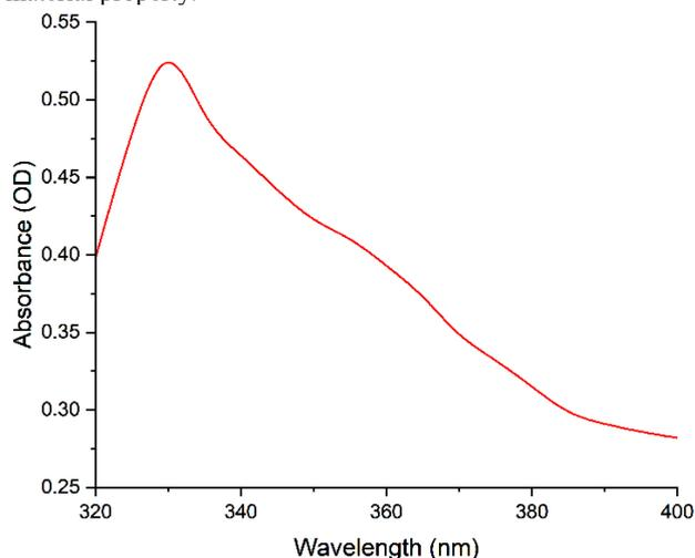
Fig. 5. UV-vis spectrum ZnO-APO paint
