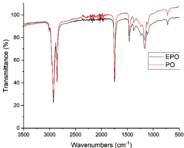
Fig. 2. FTIR spectrum of PO and EPO.
