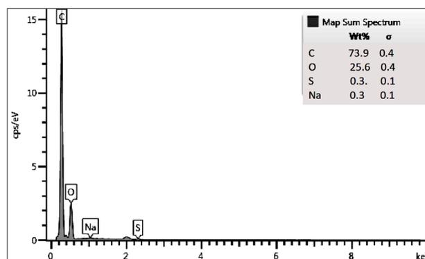
Fig. 8. EDX spectra of ZnO-APO paint.
