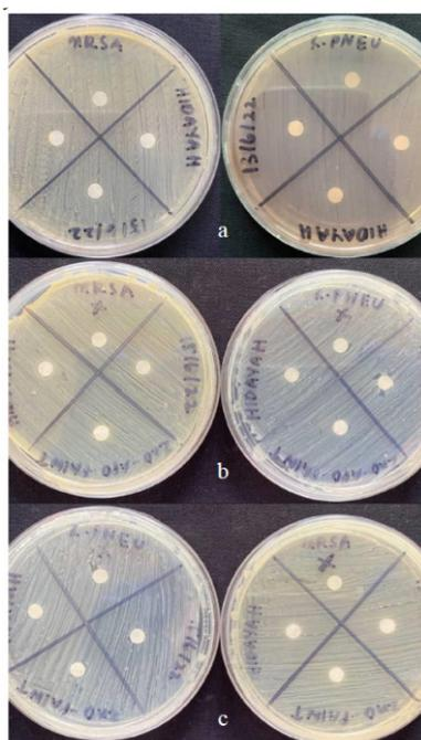
Fig. 9. Antibacterial activity test (a) ZnO-APO paint, 100 ppm (b) ZnO-APO paint, 200 ppm (c) commercial ZnO nanomaterials.
