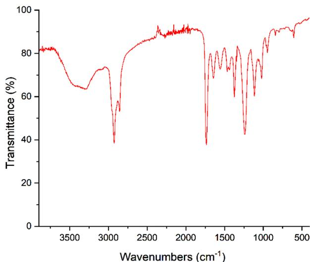
Fig. 4. FTIR spectrum of ZnO-APO paint.
