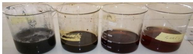
Fig. 5. Chitosan-silver nanoparticle preparations synthesized using different nominal silver nitrate concentrations.
