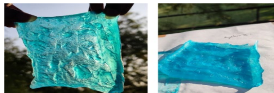
Fig. 2. Biofilm made of 10% (w/v) starch with 15% (v/v) glycerol as plasticizer with 1% (w/v) citric-acid as co-plasticizer.
