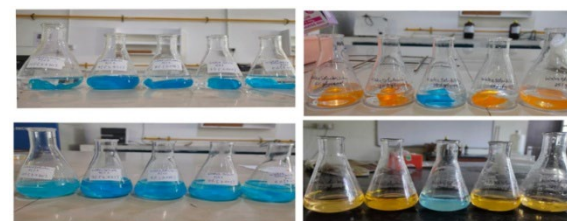
Fig. 9. Water Solubility test of different starch (w/v) % and glycerol concentrations (v/v) %.
