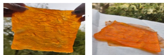
Fig. 3 Biofilm made of 10% (w/v) starch with 20% (v/v) glycerol as plasticizer with 1% (w/v) citric acid as co-plasticizer.
