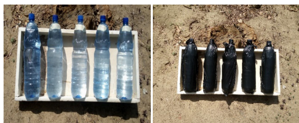
Fig. 2. Application of SODIS in household water purification. (a) Unwrapped and (b) wrapped with black plastic sheet.
