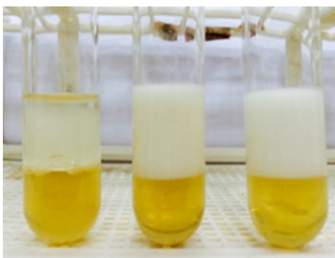
Fig. 3. Emulsification index (E24%) for treatment IV against, from left, sunflower oil, diesel and kerosene after 24 h of fermentation.
