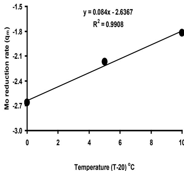
Fig. 3. Estimation of theta value for rate of Mo-reduction within the temperature range of 20 to 30 °C.
