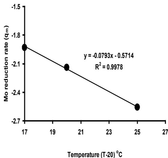
Fig. 4. Estimation of theta value for rate of Mo-reduction within the temperature range of 37 to 45 °C.
